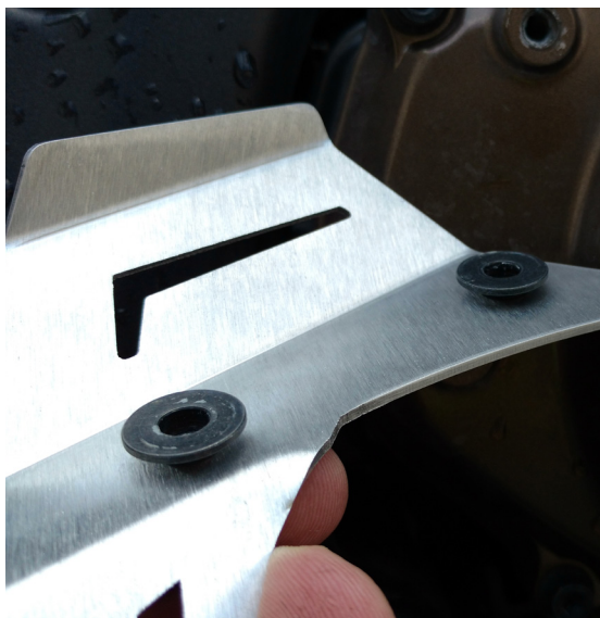
④ Arrange shoulder spacers as shown, with narrow end against the AltRider guard. Insert the screws to help hold the spacers in place.
