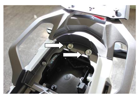
3. Use the template and drill two holes 20 mm as shown on the picture.
