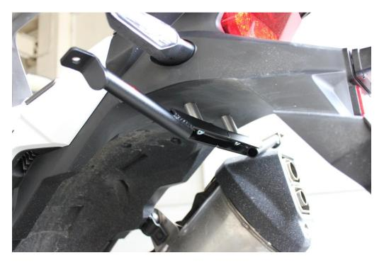
5. Put the two plastic parts on the left and right side as shown on the picture.
