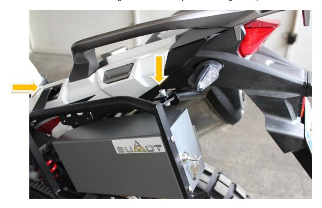
8. Attach the passenger peg with OEM bolts and washers and two spacers 20 x 7 mm and 20 x 11mm as shown on the picture. Tight them.
