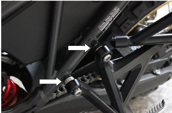
9. Install rear connecting bar with supplied M6 x 20mm bolts, M6 washers, and M6 self-locking nuts as shown below.
