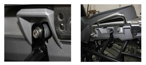
3. Now attach the pannier rack under the rear frame with M5X35 bolt and 6 mm spacer. Be carefull not to cross thread the screws.
