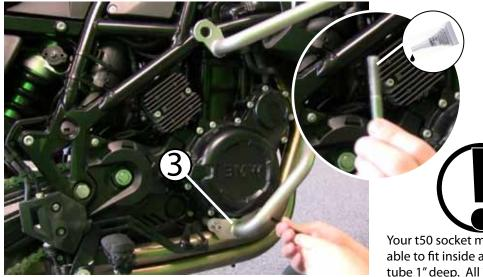
3 Use thread locker to put just one drop on the last couple threads of the (2) M8 x 60 fasteners. Now insert them with washers into the lower mount flange on the right side. Just a few turns will do!
