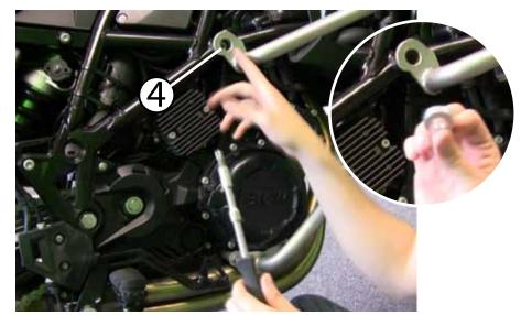
Using a T-50 torx bit, replace the OEM upper frame mount. Don't forget the spacer! Do not tighten this connection yet, just a few turns will do. You want the bar to have some wiggle room at this phase.
