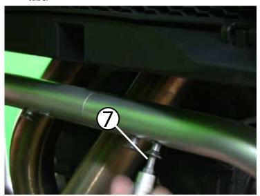
① Using a 4mm allen bit, insert the remaining (2) M6 x 20 flat head screws. Tighten these down, as well as the (2) that you put in for step one. Be careful when inserting these, you are threading into aluminum. If it feels wrong, it probably is!
