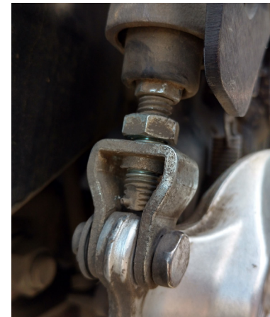
⑧ There is a limit to how much adjustment is available, make sure the plunger tip does not contact the brake lever at the very lowest height setting. Once adjusted to your preference, use the 10mm spanner to hold the shaft still, and use the 12mm spanner to tighten the nut against the yoke.
