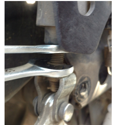
⑧ There is a limit to how much adjustment is available, make sure the plunger tip does not contact the brake lever at the very lowest height setting. Once adjusted to your preference, use the 10mm spanner to hold the shaft still, and use the 12mm spanner to tighten the nut against the yoke.
