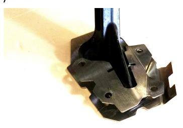
(2) Position top and bottom parts of side stand on the foot.
