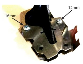
3 Place M5 x 16mm screw and one M5 x 12mm screw as shown. Get the threads started, but do not completely tighten.
