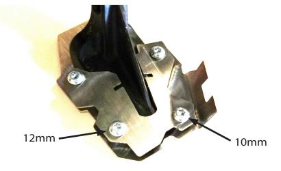
(4) Insert second M5 x 12mm screw and M5 x 10mm screw as shown. Tighten until tip of screws is flush with the bottom of the lower plate.
