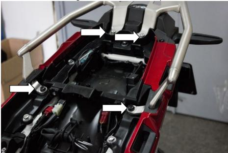
4. Remove the two bolts as shown on the picture and plastic cover
