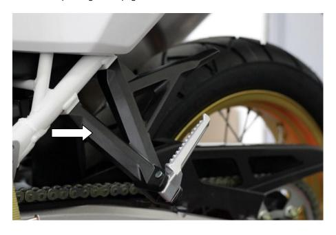
3. Remove the four bolts and grab handle as shown on the picture
