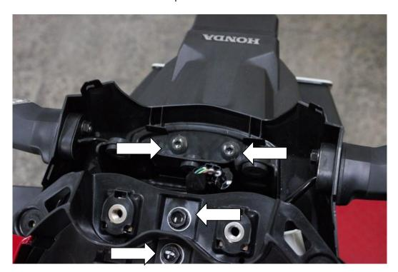
7. Remove the two bolts under the mud guard and two nuts as shown on the picture
