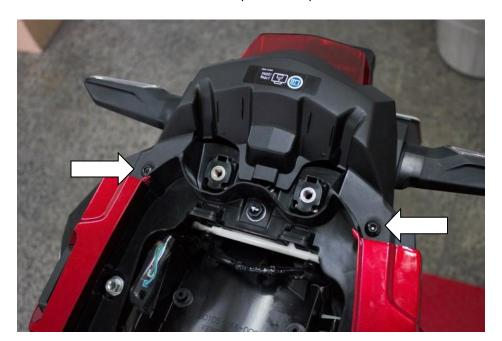
5. Disconnect the plug from the tail light and remove the two nuts and head washers as shown on the picture
