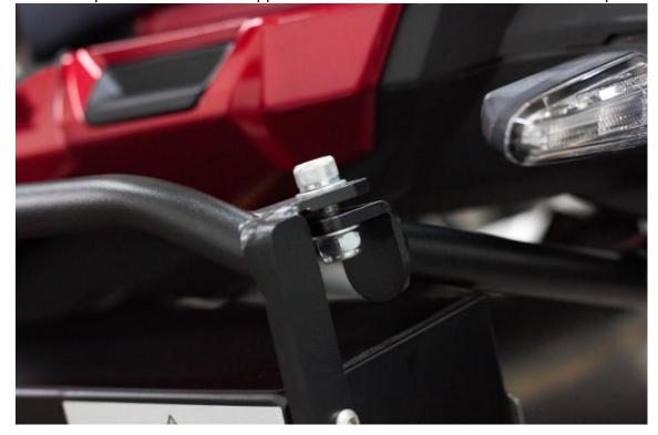
14. Attach the cross bar with M6 x 20mm as shown on the picture:
