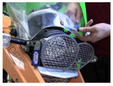
We recommend using masking tape because it will hold the nut in, while you do the rest of the install.
