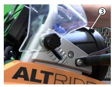
Using a T10 torx tool, remove the (2) screws that hold the headlight front bezel. (one on the left and one on the right)
