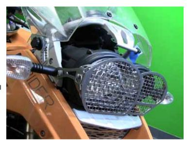
Use a T25 torx bit to remove the (2) front windscreen fasteners. You can use a little masking tape or a magnetic finger glove to hold the nut on the back side of the windscreen mounts.
