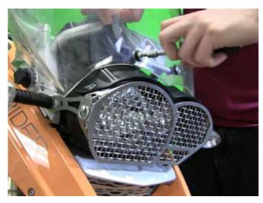
(5) Using a finger to hold the nut in place, and a T25 torx bit and driver, put the OEM fasteners back that hold the wind screen.
