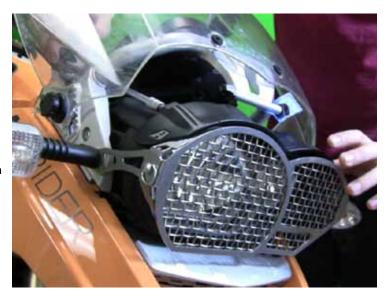
Put the Anti-glare Guard on top of the bezel. Using a T15 torx bit and an extension, attach the guard using the supplied screws.
