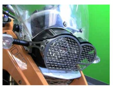
6 Check to make sure your adjustment knobs and windscreen fasteners are all tightened appropriately.
