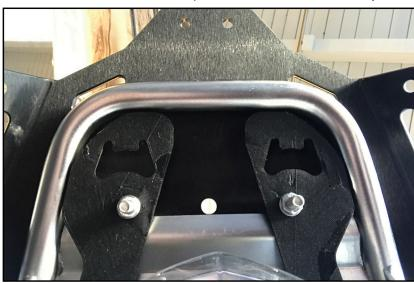
The brackets should align with the stainless tube frame as shown above.
