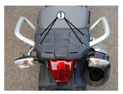
Using an 8mm socket and driver or ratchet, remove the (4) OEM fasteners that hold the plastic rack in place. Keep in a safe place (we recommend a labeled bag or bin) you will not be re-using these.
