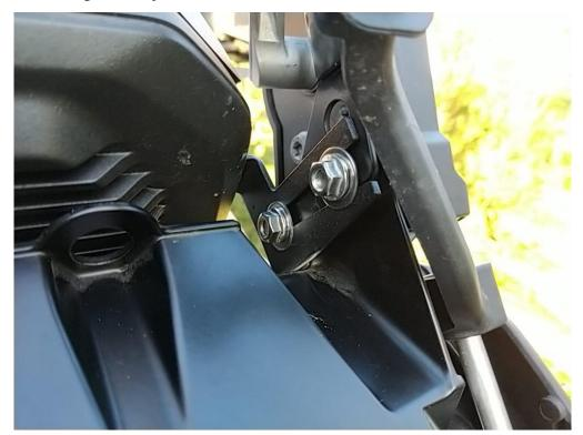
Fit the M6 washers and the nuts. approach the nuts without blocking, place your protection correctly then moderately block the nuts (a little medium thread lock does not harm).
