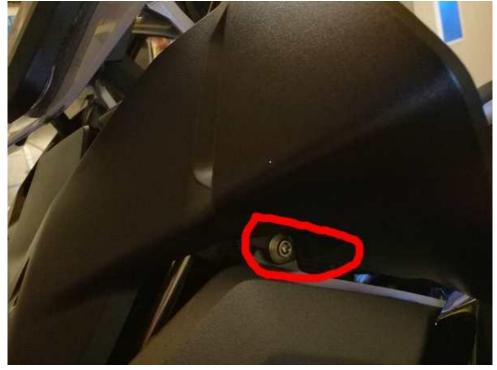
Remove the 4 screws (2 on each side) which also hold the GPS support by replacing them with the 4 screws supplied M6 X 25.
